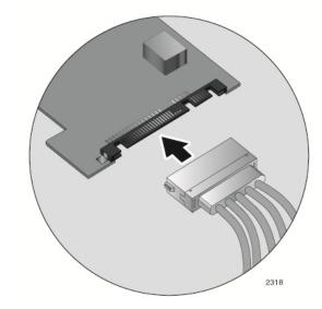
Figure 7. Installing System PS SATA Harness connector to AT-2716POE
